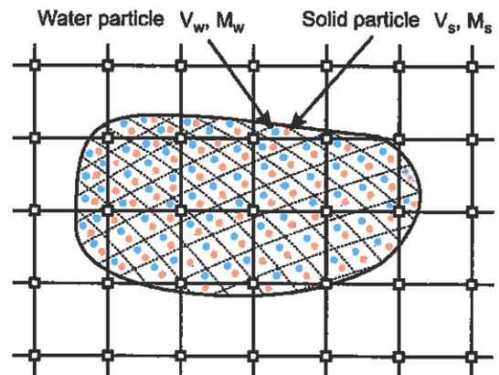
Figure 3: Discretization of MPM using two particle sets
