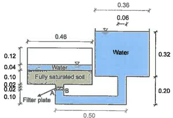
Figure 6: Geometry of the MPM model for hydraulic heave problem (all dimensions in meter)
