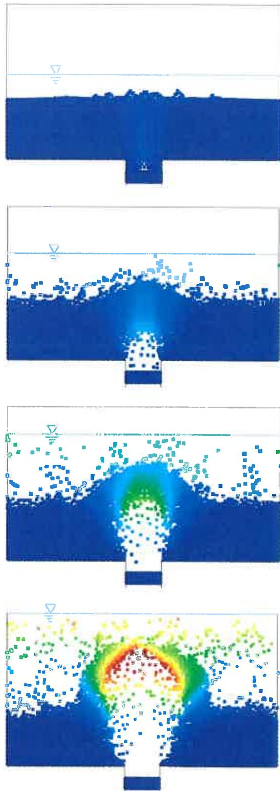
Figure 7: Displacement of soil grains at different time stages where the water particles are turned off to focus on the behaviour of sand (dark blue zero with dark red 0.216 [m])
