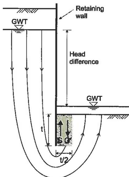
Figure 1: Hydraulic heave with Terzaghi's approach
