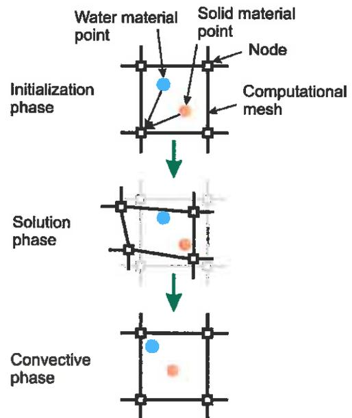
Figure 2: Working procedure of MPM
