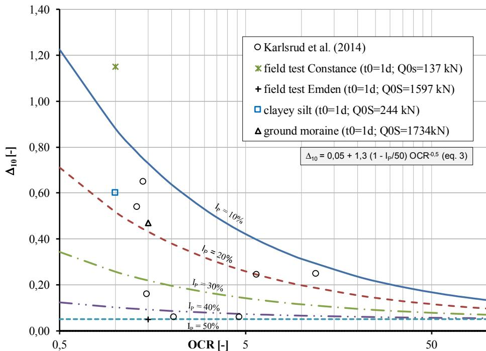
Figure 7: Connection of set-up, over consolidation ratio and plasticity index
