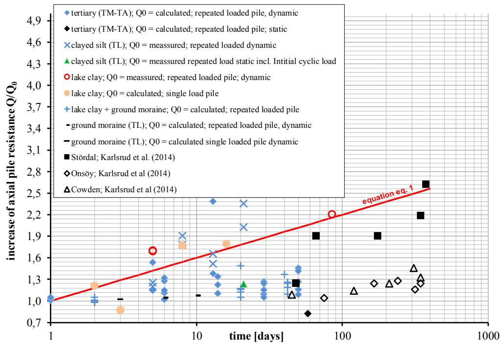
Figure 6: Data of project based load tests on precast driven piles in cohesive soil
