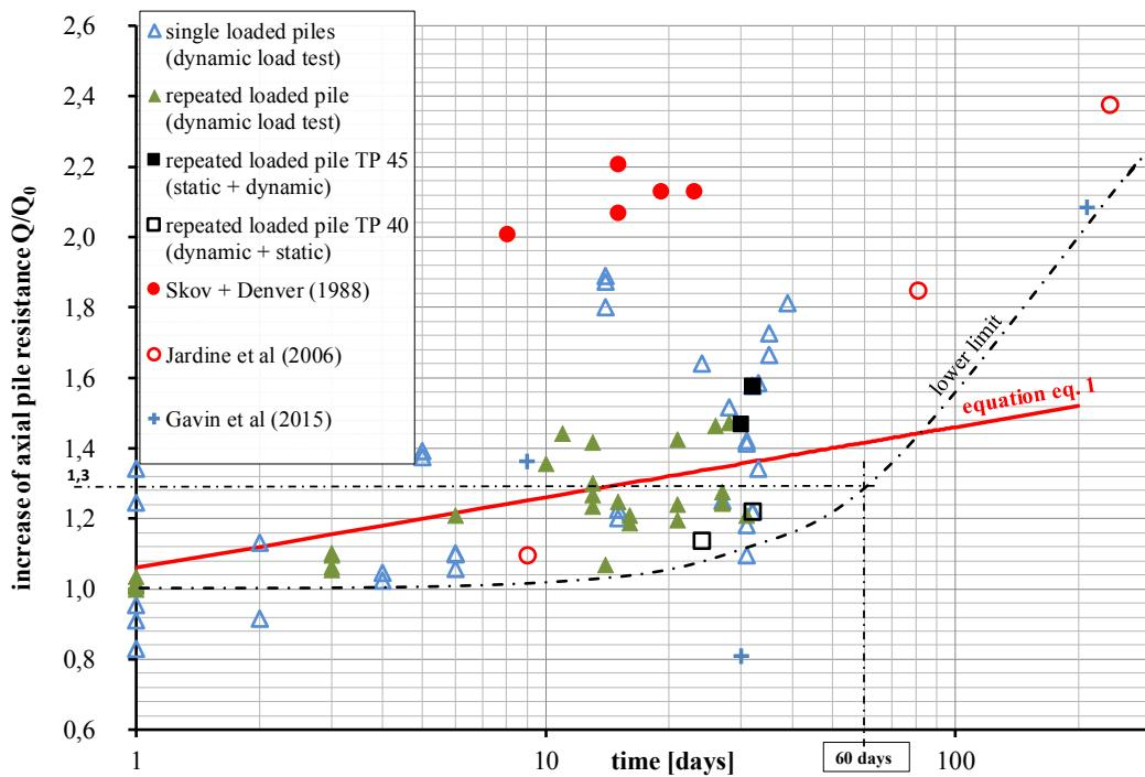
Figure 5: Data of project based load tests on precast driven piles in sands
