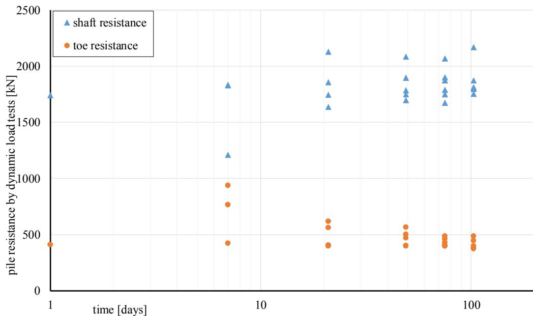
Figure 4: Results of dynamic load tests separated in shaft and toe resistance
