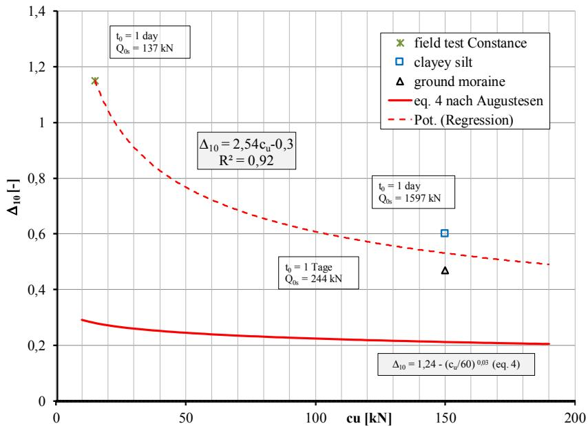
Figure 8: Connection of set-up and undrained shear strength
