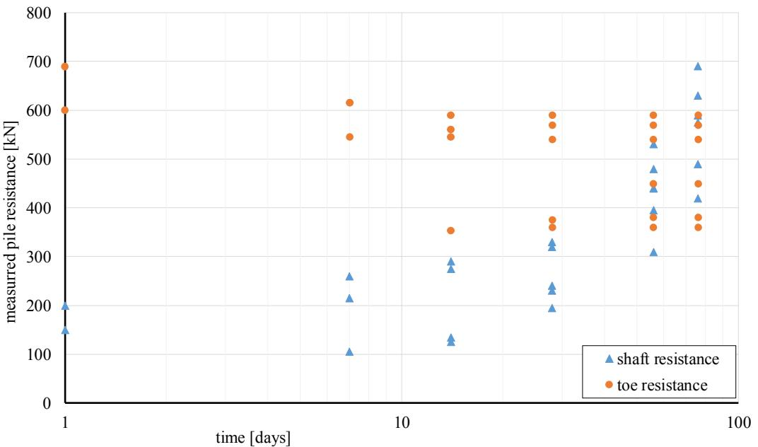
Figure 2: Results of dynamic load tests separated in shaft and toe resistance
