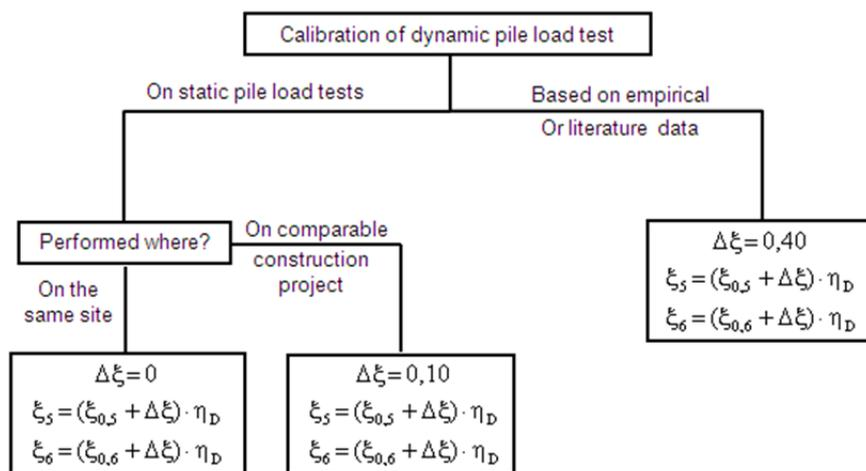
Figure 11: Procedure for deriving the correlation factors  $\xi_5$  and  $\xi_6$  for dynamic pile load tests as a function of the calibration based on Table 12
