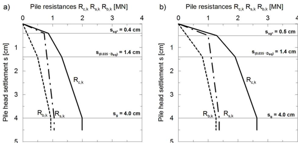
Figure 18: Resistance-settlement curve; a) Lower values, b) Upper values
