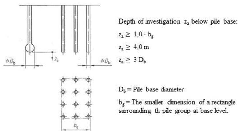
Figure 2: Minimum ground investigation depths for pile foundations, from EC 7-2 Handbook (DIN 2011b); Note: if the pile resistances of compression pile foundations are determined based on data from proven experience acc. to 'EA-Pfähle', the ground investigations should extend to a depth below the pile base of at least  $z_a \geq 4D_b$
