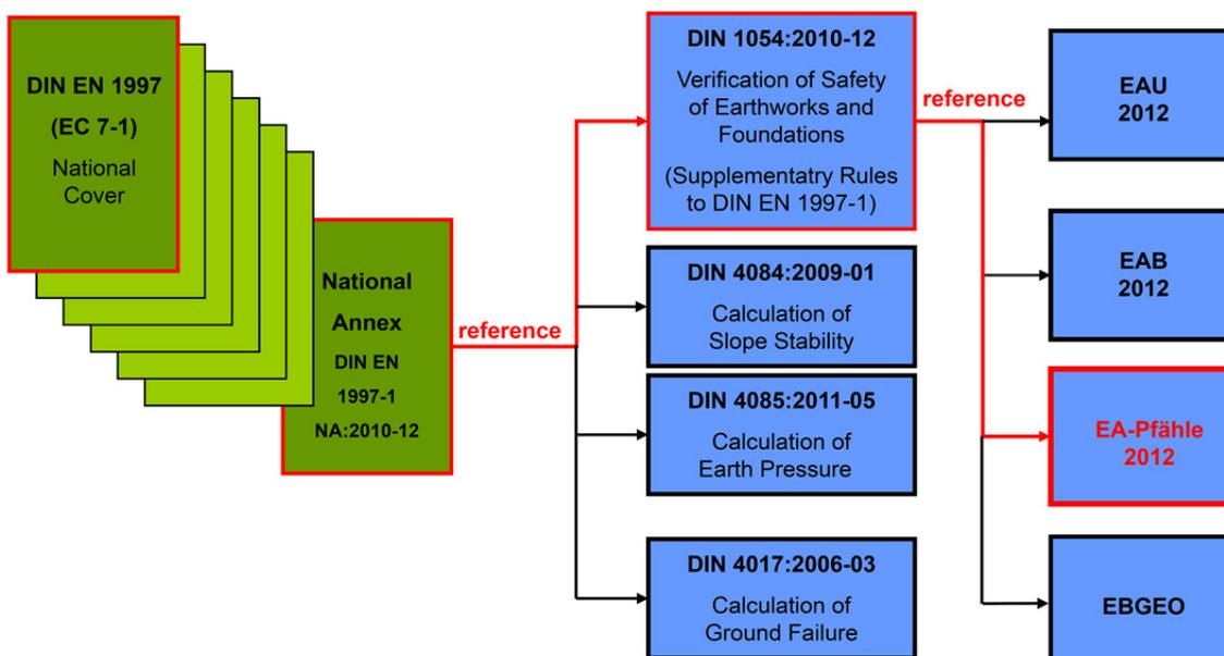
Figure 4: Overview of European and national standards and recommendations for pile design in Germany
