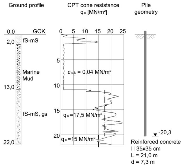
Figure 17 Ground profile, penetration test diagram and dimensions for an example calculation for the resistance-settlement curve
