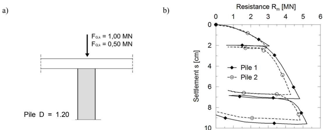
Figure 12 a) System and effect; b) Logged  $R_m$  values for both static pile load tests
