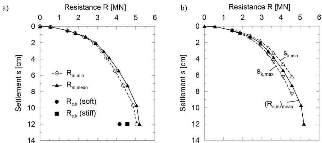
Figure 13 a) Characteristic pile resistances in the ultimate limit state (ULS) for piles of "flexible" and "stiff" structures derived from the  $R_{m,i}$  values recorded in static pile load tests; b) Section of the resistance-settlement curves in the serviceability limit state (SLS) and derivation of characteristic boundary curves
