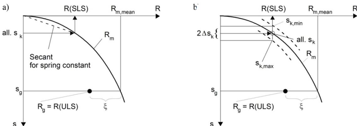
Figure 9: Possible method for derivation of characteristic resistances of isolated piles  $R(\text{SLS})$  in the serviceability limit state from test data and data from resistance-settlement curves a) for anticipated minor differential settlements between isolated piles; b) for anticipated substantial differential settlements between isolated piles
