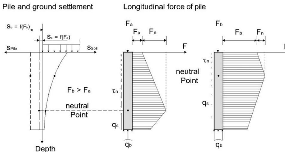
Figure 8 Qualitative relationships between pile resistances and effects from structural loads, and negative skin friction in homogeneous ground, and the definition of the neutral point.
