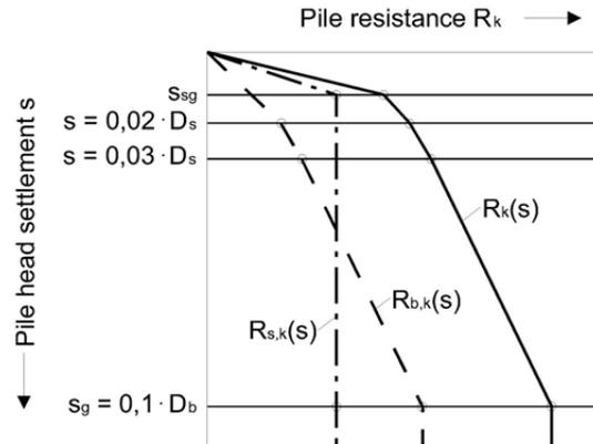
Figure 7: Elements of the characteristic resistance-settlement curve for bored piles
