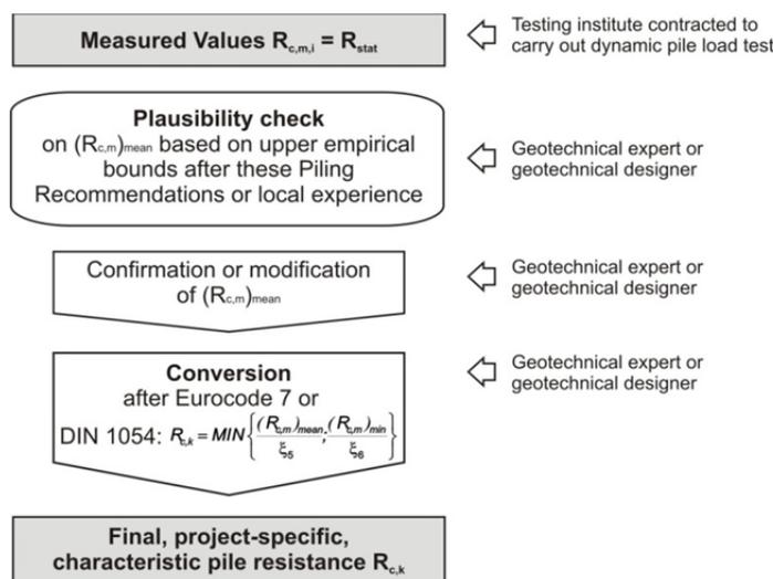
Figure 10: Steps to determine characteristic pile resistances from measured or test data of dynamic pile load tests
