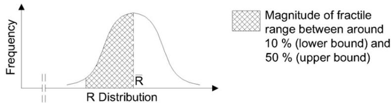
Figure 6: Fractiles for the ranges of pile resistance table data from empirical data, compared to load test results
