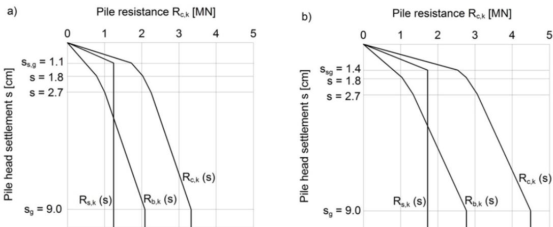
Figure 16: Resistance-settlement curve; a) Lower values, b) Upper values
