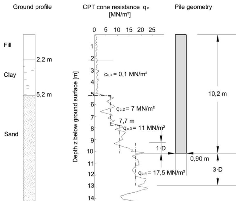
Figure 15: Ground profile, penetration test diagram and dimensions for an example calculation of the resistance-settlement curve;  $D = 0.9 \text{ m}$ ,  $U = 2.83 \text{ m}$ ,  $A = 0.64 \text{ m}^2$
