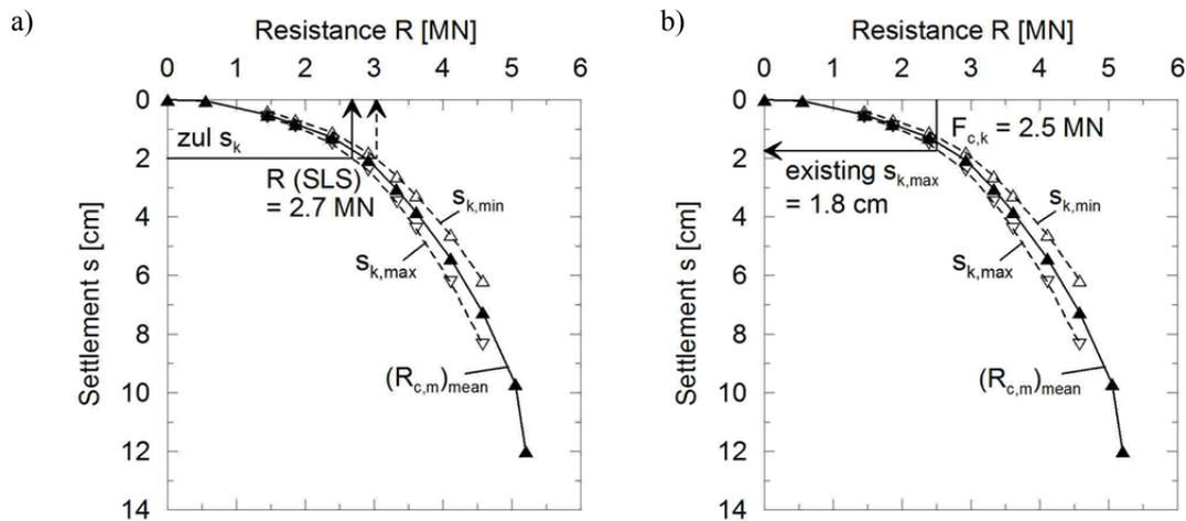
Figure 14 a) Analysing serviceability via the characteristic pile forces; b) Analysing serviceability via existing and allowable settlements
