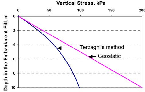
**Figure 3.3: Typical vertical stress distribution of embankment fill between trap-door with Terzaghi's method**
