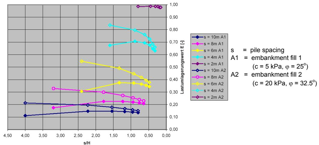
Figure 4.3: The change of efficacy to the ratio of spacing to embankment height (Sovulj, 2005)
