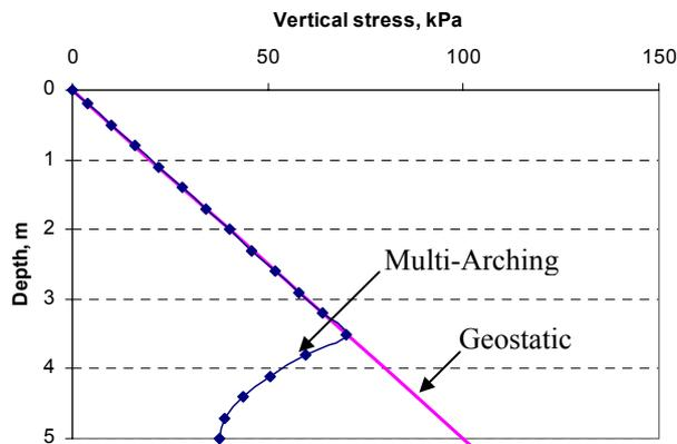
Figure 3.9: Typical vertical stress distribution of embankment fill along the centre of pile spacing with Multi-Arching model
