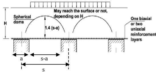
Figure 3.5 Arching dome according to British Standard (Alexiew, 2004)
