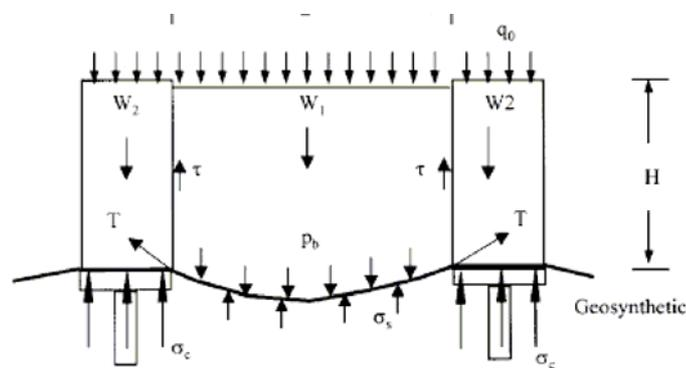
Figure 4.1: Load transfer mechanisms of piled embankments
