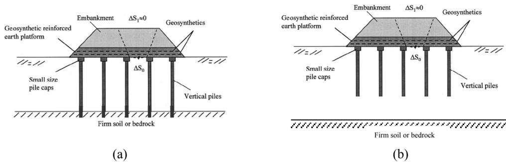
**Figure 2.1: Piles-supported embankment (a) on end bearing piles (b) on floating piles**
