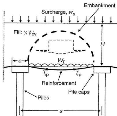
Figure 3.10: General idea of geosynthetic reinforcement (BS 8006)
