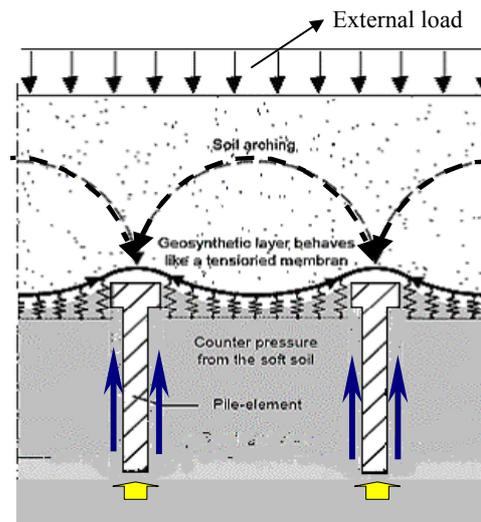
**Figure 3.1: The Idea of Piled Embankment**
