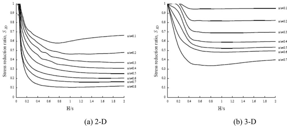
**Figure 4.6: The comparison between 2-D plane strain and 3-D analyses (Kempton et al., 1998)**
