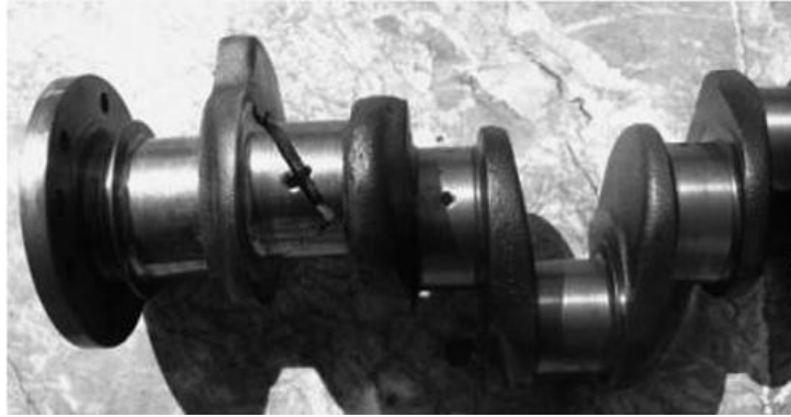
Figure 1. Crack propagation in the crankshaft [10].
