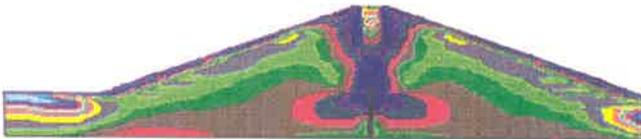
Shading of relative shear stress ( $\tau/\tau_{max}$ )
