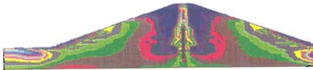
Shading of relative shear stress ( $\tau/\tau_{\max}$ )
